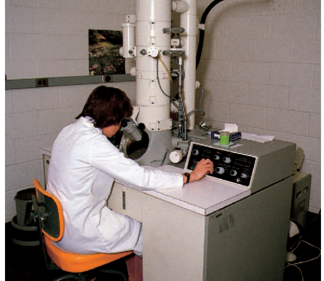
Figure 2.22 A Modern Transmission Electron Microscope. The electron gun is at the top of the central column, and the magnetic lenses are within the column. The image on the fluorescent screen may be viewed through a magnifier positioned over the viewing window. The camera is in a compartment below the screen.
