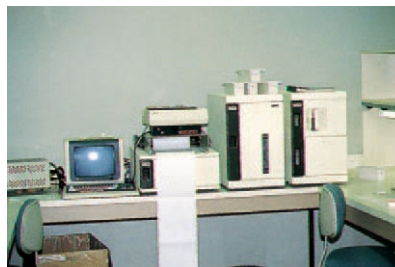
(h) In a short period of time, sometimes 4 hours, computer-generated information is obtained that will consist of biochemical identification and antibiotic susceptibility results.
