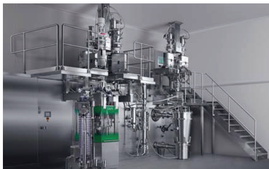
Fig. 34.10 The GEA ConsiGma, a continuous manufacturing line for the manufacture of tablets via twin-screw wet granulation. (Reproduced from https://www.gea.com/ .)
