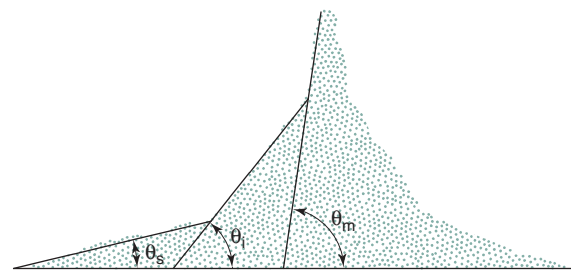
Fig. 12.1 Cohesive powder poured in a heap and showing different angles of repose: \theta_m , maximum angle formed by cohesive particles; \theta_s , shallowest angle formed by collapse of the cohesive particle heap, resulting in flooding. In some cases, a third angle, \theta_i , is identifiable as an intermediate slope produced by cohesive particles stacking on flooded powder.
