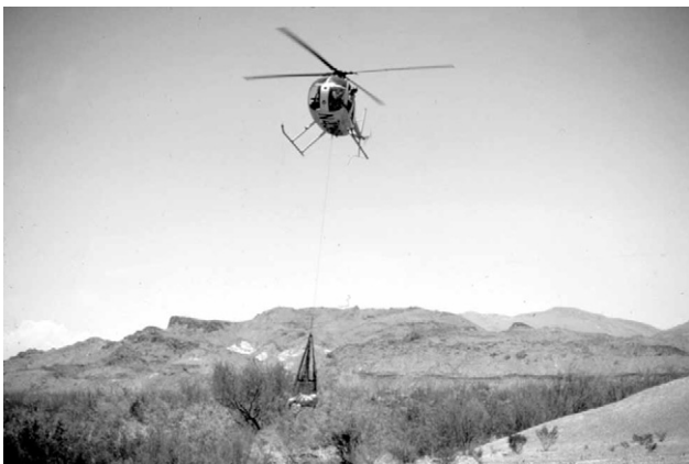
FIGURE 7 A helicopter carries bags of sediment for screening from a remote part of Big Bend National Park.
