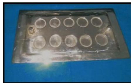
FIGURE 1: Metallic mold used for fabricating the heat-cured acrylic samples.
